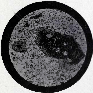
FIG. 2.—FROM SECOND PERIOD STREAM (WELL DIGGING), SHOWING HORNBLLENDE COMPLETELY ALTERED TO AUGITE OPACITE AGGREGATE.
